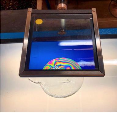
This image is looking at a stressed glass work under PGC's polariscope. Although the stressed glass looks beautiful and colorful under the polariscope the object is likely to break.
