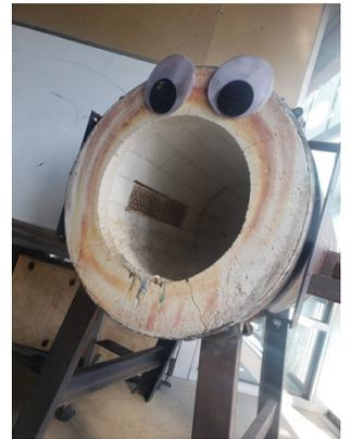
Roary is one of our many reheating chambers, also known as a "glory hole." The glory hole is a metal drum turned on its side, lined with a high-temperature refractory brick and material. It is powered by natural gas and resides at around 2150°F at working temperature. Glory holes are only turned on as needed, but need about half an hour to warm up before working.
